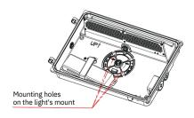
8.Usescrew to lock the lamp base on the embedded junction box, and ensure the balance of the horizontal column.
