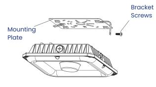
1. Unscrew the bracket screws and remove the mounting plate from the lamp housing.
