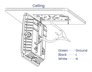
3. Insert the clip ring of the plate into the latch of the light fixture housing, and hang the fixture on the bracket.
