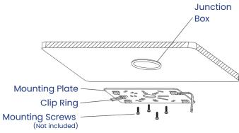
2. Secure the mounting plate to the ceiling using screws.
